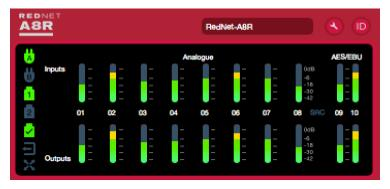
The illustration above shows a RedNet A8R with signals present on all input and output channels. The unit has a single PSU input, single network input and a locked network connection.
