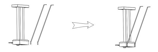
D) Then reserved the Pedal component with two copper poles(I), and use the hexagonal bolt(G) to tightly settled it with the piano body according finished assembly in left leg component, fix the other side of copper Pole onto the piano body (E). The assembly are finished. (See the below illustration.)
