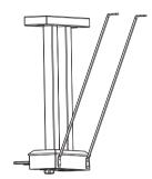
D. Then reserved the Pedal component with two copper poles(I), and use the hexagonal bolt(G) to tightly settled it with the piano body according finished assembly in left leg component, fix the other side of copper Pole onto the piano body (E). The assembly are finished.
