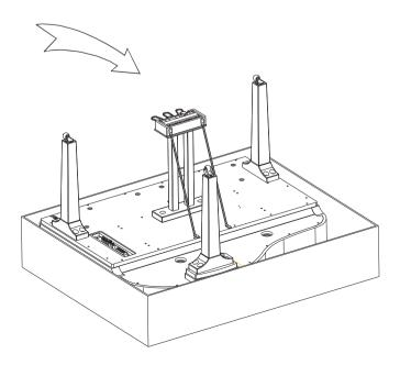
E. Reverse the piano after finished assembly. Please carefully reverse the piano avoid touched floor cause damaged or broke any leg components or pedal component. Then moved the carton box and all package goods. You can enjoy play the piano now.
