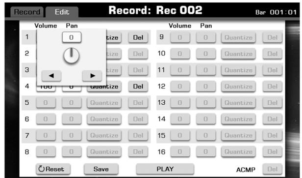
Press the “Quantize” button to call up a pop-up box showing the quantize accuracy. Use the DATA DIAL, the [+] or the [-] button to adjust the parameter. Press “OK” to confirm executing quantize.
