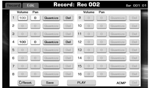
Press the Volume “100” button to call up a pop-up box showing the adjustable range of volume values. Use the DATA DIAL, the [+] or the [-] button to adjust the volume.
