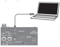
\* Use a commercially available USB 2.0 cable to make this connection.
